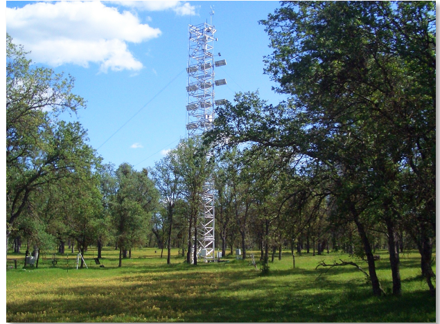
Figure 6. Evapotranspiration is measured directly via the eddy covariance technique from instruments attached to towers extending above canopies, which allows for relatively large-scale integrated measurements over ~1 km footprints.
