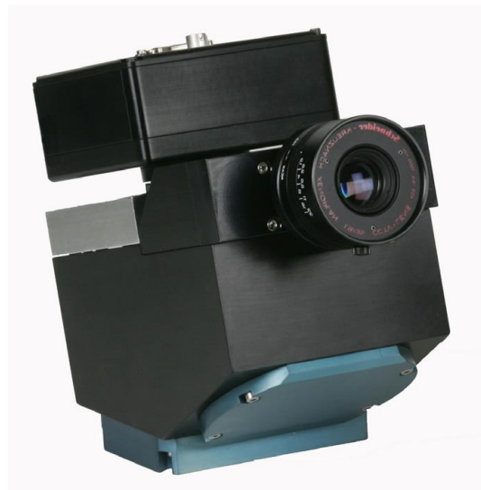
Figure 6. Operating specifications for the Hyperspec™ VNIR Concentric Imaging Spectrometer manufactured by Headwall Photonics, Fitchburg, MA. FOV = 2\arctan(d/2f) = 49.64 deg, where f=8 mm lens and d=7.4 mm.
