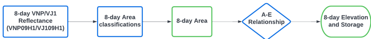
Figure 1. Flow chart of the algorithm for deriving the VNP28C2/VJ128C2 product, which contains 8-day area, elevation, and storage results for the 164 reservoirs. The product components are shown in green boxes.
