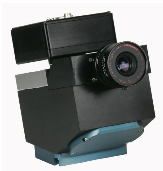
Figure 6. Operating specifications for the Hyperspec™ VNIR Concentric Imaging Spectrometer manufactured by Headwall Photonics, Fitchburg, MA. FOV = 2\arctan(d/2f) = 49.64 \text{ deg} , where f=8 \text{ mm} lens and d=7.4 \text{ mm} .
