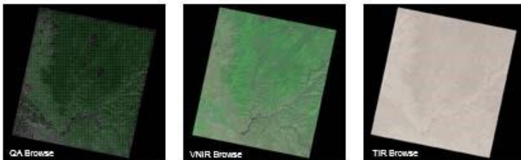
Figure 3. AST_L1T QA browse, VNIR full resolution browse, and TIR full resolution browse GeoTIFF images
