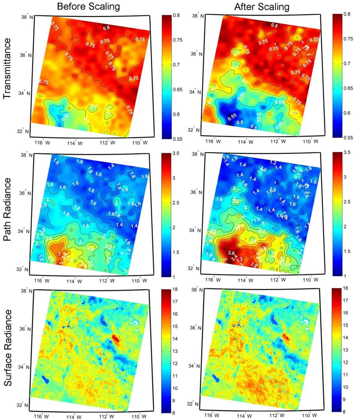
Figure 5. Comparisons between the atmospheric transmittance (top), path radiance ( $W/m^2/\mu m^{-1}$ ) (middle), and computed surface radiance ( $W/m^2/\mu m^{-1}$ ) (bottom), before and after applying the WVS scaling factor  $\gamma$  to a MODIS scene cutout shown in Figure 5. Results are shown for MODIS band 29 ( $8.55 \mu m$ ).
