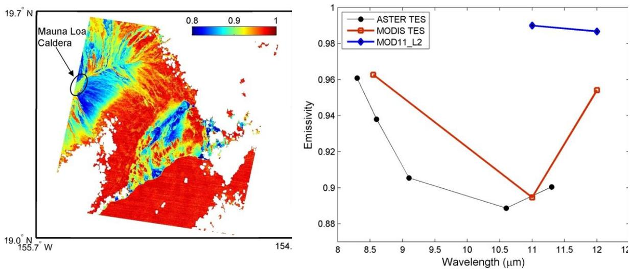
**Figure 18. (left) ASTER band 12 (9.1  $\mu\text{m}$ ) emissivity image over Mauna Loa caldera, Hawaii on 5 June 2000, and (right) emissivity spectra from ASTER, MODTES, and MOD11 emissivity classification. While ASTER and MODTES agree closely, MOD11 emissivities are too high, resulting in large LST discrepancies between MODTES and MOD11 (12 K) due to misclassification in bands 31 (11  $\mu\text{m}$ ) and 32 (12  $\mu\text{m}$ ).**
