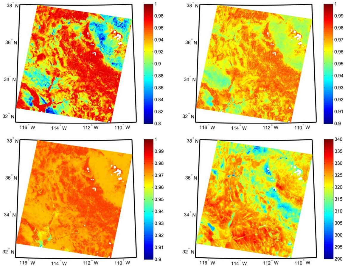
Figure 13. Clockwise from top left: MODIS cutouts of land surface emissivity for band 29 (8.55  $\mu\text{m}$ ); band 31 (11  $\mu\text{m}$ ), band 32 emissivity (12  $\mu\text{m}$ ), and LST output from the TES algorithm over the Imperial Valley, southeastern California on 29 August 2004.
