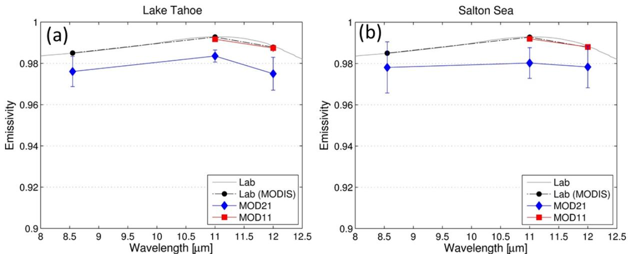
**Figure 22. Figures showing the Emissivity retrievals for the MODIS Aqua MYD21 products over two water sites using data collected for three years of data for Lake Tahoe (2003-2005) and Salton Sea (2008-2010). Lab data, Lab data convolved with MODIS bands and the MOD11 bands 31 and 32 are also shown for comparison.**
