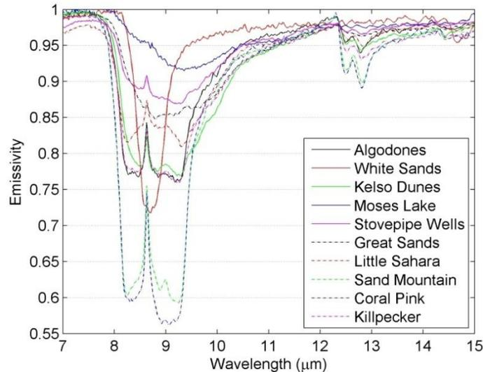
**Figure 24. Laboratory-measured emissivity spectra of sand samples collected at ten pseudo-invariant sand dune sites in the southwestern United States. The sites cover a wide range of emissivities in the TIR region.**
