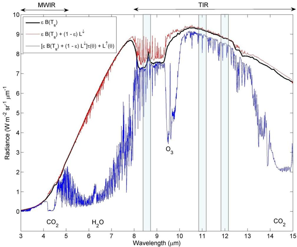
**Figure 2. Radiance simulations of the surface-emitted radiance, surface-emitted and reflected radiance, and at-sensor radiance using the MODTRAN 5.2 radiative transfer code, US Standard Atmosphere, quartz emissivity spectrum, surface temperature = 300 K, and viewing angle set to nadir. Vertical bars show placements of the MODIS TIR bands 29 (8.55  $\mu\text{m}$ ), 31 (11  $\mu\text{m}$ ), and 32 (12  $\mu\text{m}$ ).**
