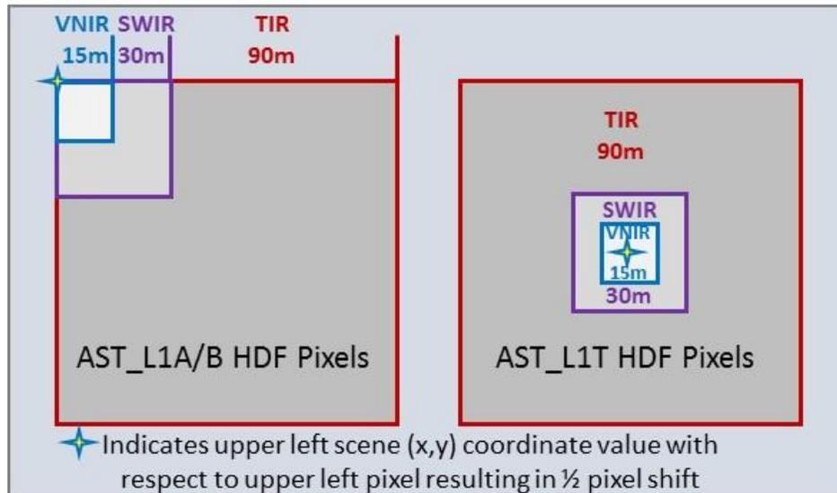
**Figure 2-3. Pixel Centering for AST\_L1A/B and AST\_L1T Bands.**
