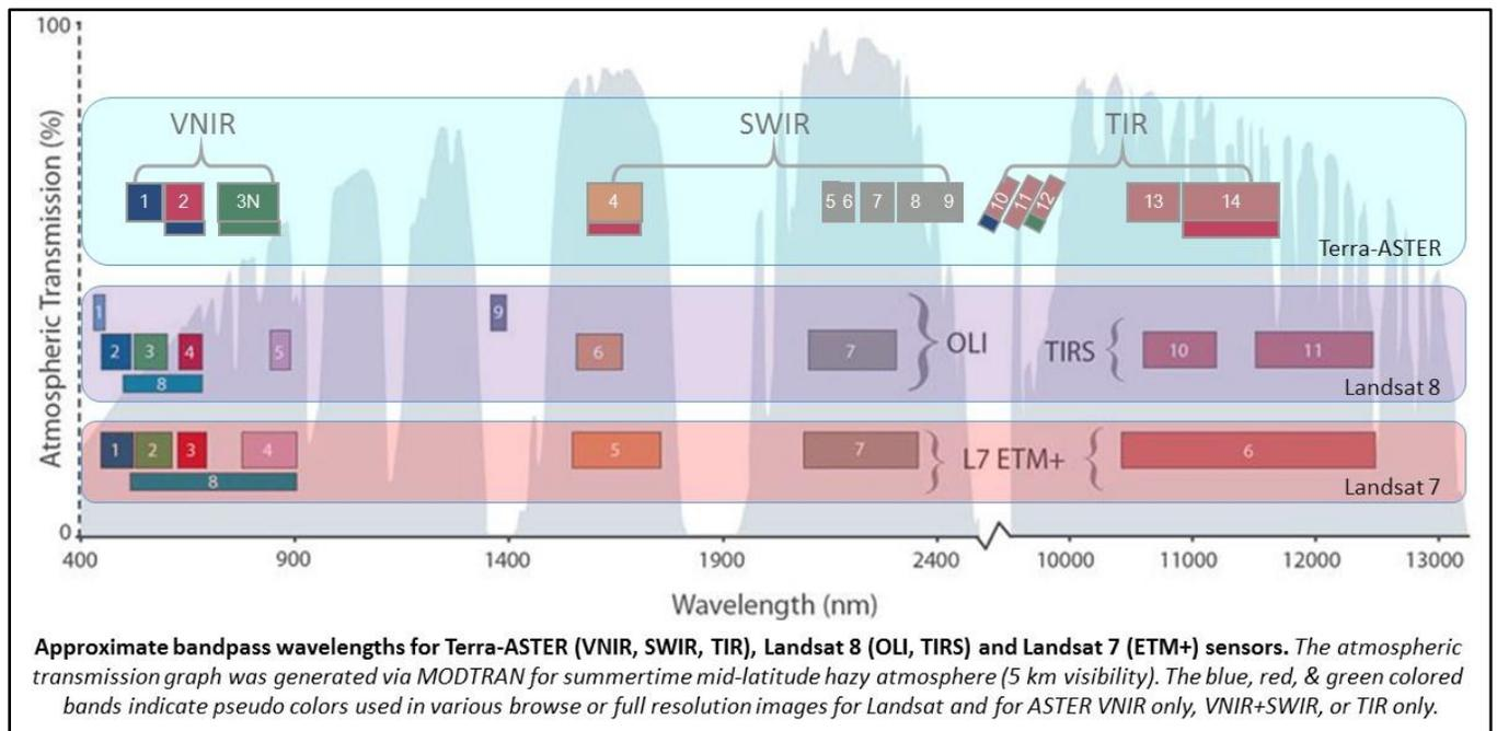
**Figure 1-1. Terra ASTER and Landsat 7/8 Spectral Bands Compared.**
